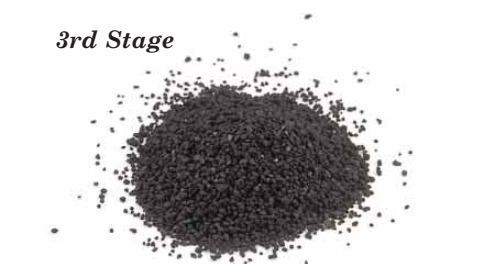
Activated carbon filter removes mercury vapors released during crushing.
